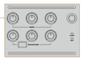
The color balance controls let you make fine adjustments to the red, green, blue channels for the master gain/white, gamma and pedestal/black levels
