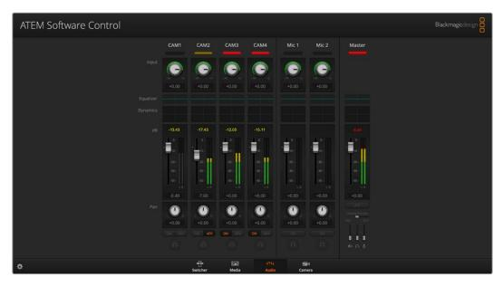
Your ATEM Mini also features built in mic inputs for mixing external audio.
