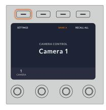
Press the 'settings' soft button on the LCD home screen to access all the camera control panel's settings
