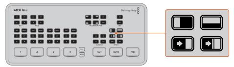
Press the transition type button for the transition you want to use, for example a horizontal or vertical wipe, push or squeeze DVE transition, and mix or dip transition
