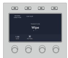
Press a source button in the source select row to select a source for the wipe border. Hold the shift button down to select a shifted source, such as a color generator or media player.
