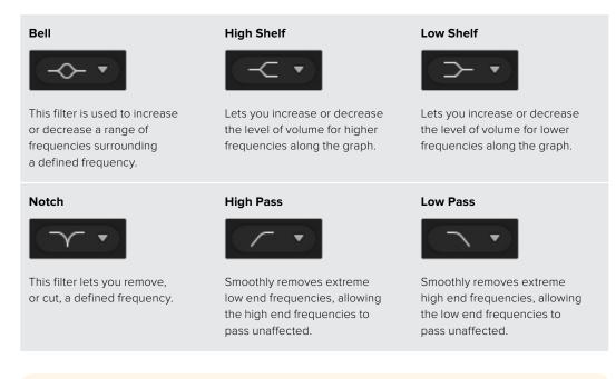
**TIP** It's not uncommon to have filters on each band overlapping on the graph curve with adjustments working together. For example, you may have a low shelf filter applied to band 4, and a notch filter on band 5 reducing a frequency within the same range.
