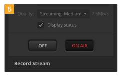
With all the streaming details now set, it's worth performing a quick test broadcast to make sure everything is working. Press the 'on air' button on ATEM Mini Pro, or click on the on air button in the live stream palette.
