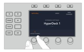
As HyperDecks must buffer a couple of frames before commencing playback, the actual cut will be delayed a preset number of frames to ensure a clean transition. This is just like setting a preroll on a videotape machine. You can adjust the length of this delay by changing the 'offset' frames number using the control knob under this indicator. Press the soft button above the 'save changes' indicator to confirm your change.
