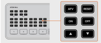
To enable or disable AFV for each input, simply press its AFV button.
