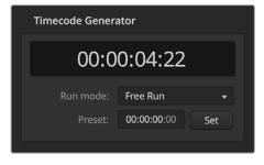
When using ATEM Mini Pro, the timecode generator can be set to time of day, or free run timecode where you can set a manual preset timecode
