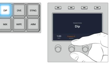
Press the 'dip' button in the transition control block, then set the dip source and transition rate using the LCD menu
