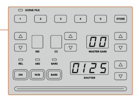
The upper section of each CCU is used to store and recall scene files, plus control camera settings such as shutter speed, master gain, white balance and color bars
