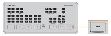
To fade up from black, simply press the FTB button again. This is a clean way of starting and finishing a broadcast.
