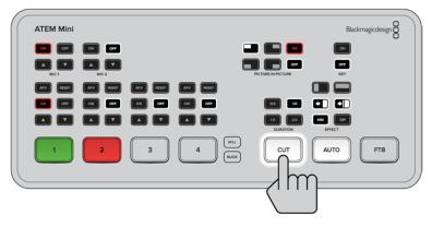
In program preview switching mode, press an input button and then press the 'auto' or 'cut' button to switch the source to air
