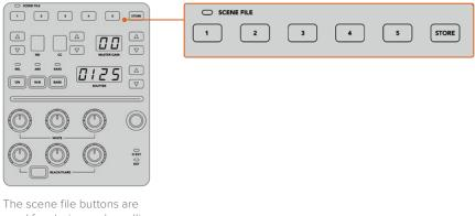
used for storing and recalling all settings for CCU controls
