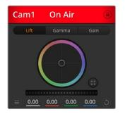
Each camera controller displays the channel status so you know which camera is on air. Use the color wheels to adjust each YRGB channel's lift, gamma and gain settings.
