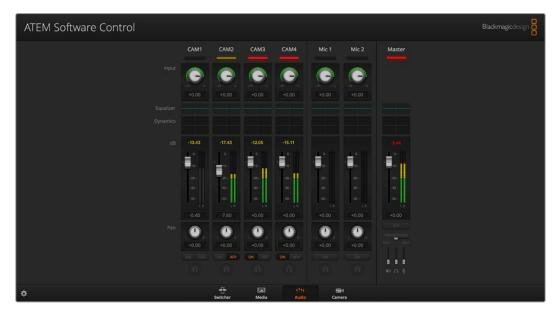
The audio mixer displays tally lights for any audio sources that are currently on air or when AFV is selected, as well as audio level, audio balance and buttons for selecting which audio should be used
