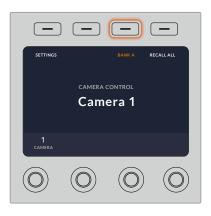
Press the bank soft button to cycle between camera banks A and B, or hold the button down to disable or enable camera banks
