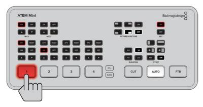
In cut bus mode, pressing an input button will instantly switch it to air
