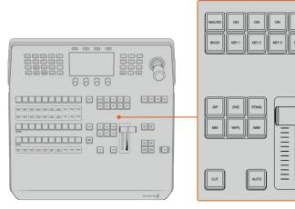
Press the button marked CUT in the transition control block to perform a cut transition
