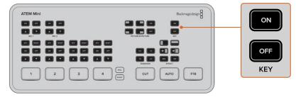
Press the 'key' on or off buttons to switch the upstream keyer on and off air
