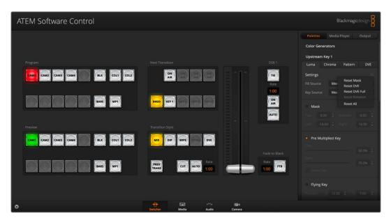
ATEM Software Control is included in the ATEM sotware installer and can be downloaded from the Blackmagic Design website. It's free and allows you to control your switcher in a similar way to a full hardware control panel. A range of palettes on the right side shows you all processing features of your ATEM Mini and allows settings to be easily made.
