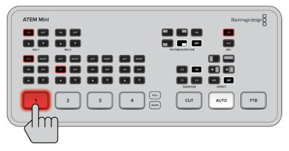
ATEM Mini's control panel lets you switch video sources, adjust audio levels, perform transitions and apply graphics and effects
