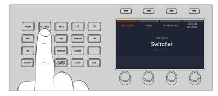
You'll notice that ATEM 1 M/E Advanced Panel displays four setup options along to top of the LCD screen. These include 'switcher,' 'panel,' 'HyperDecks,' and 'button mapping.' Each corresponds to a setup menu. Simply press the LCD soft button above 'HyperDecks' to enter the 'HyperDeck settings' menu.
