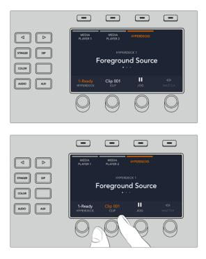
You can now use the rotating knobs below the 'hyperdeck,' 'clip,' 'jog' and 'shuttle' indicators to select HyperDecks, select clips, and jog and shuttle these clips.
