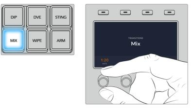
Press the 'mix' button and set the transition rate using the LCD menu
