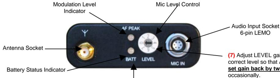
(4) Switch on TX (by connecting microphone cable to 6-pin LEMO socket)
