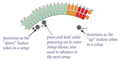
The mixer will not pass audio when in the Setup Menu. When in the Setup Menu the flashing LED on the left meter (L) position indicates the selected setup feature. The right meter (R) position indicates the values selected for the setup. Use the PK/VU button advance from one setup to another. If the intended setup is passed, setup mode must be re-entered since you can only step forward through the Setup Menu.
