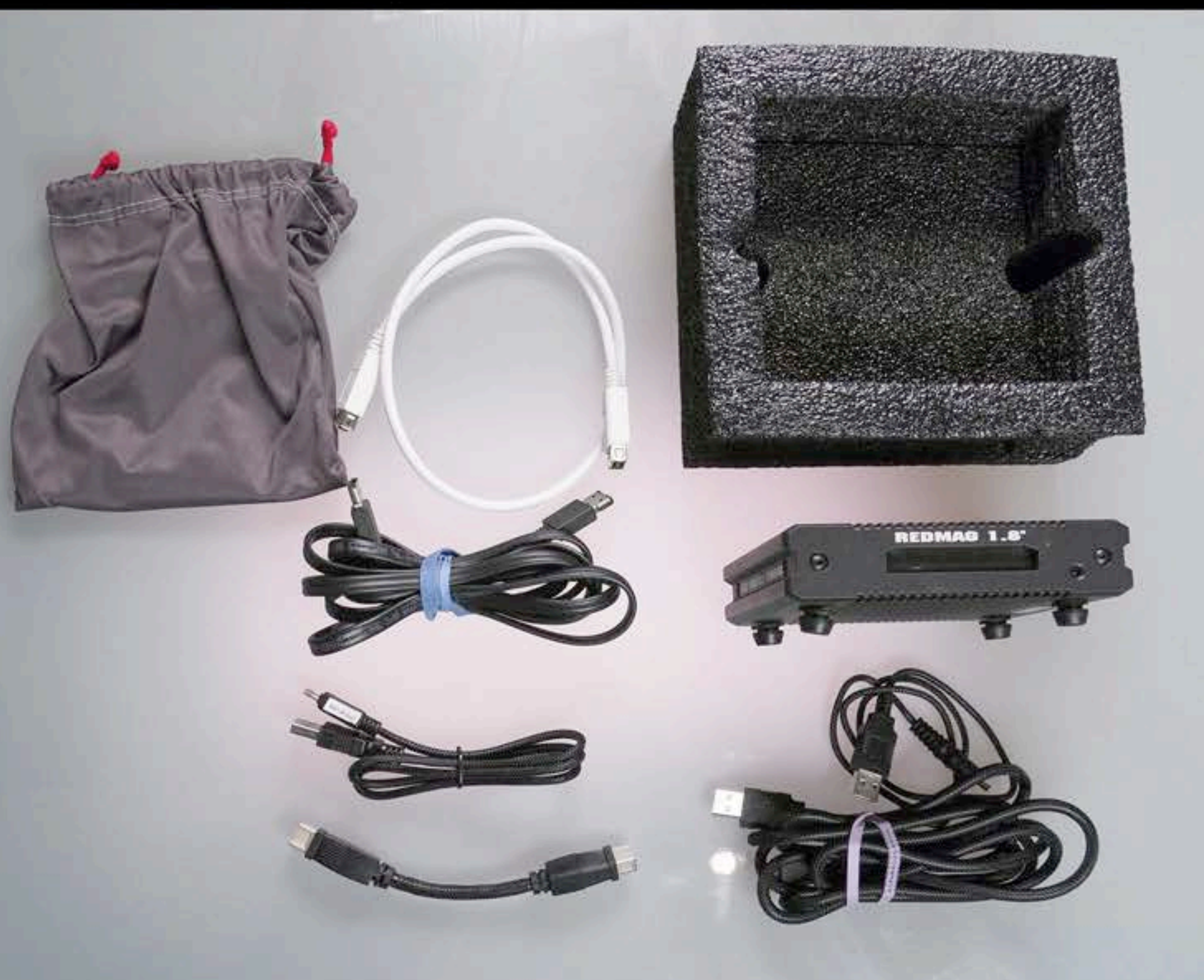
REDMAG driveeSata Cable, Firewire 800 to 800 ca USB A to mini B, USB to DC power, Velvet pouch for cables
