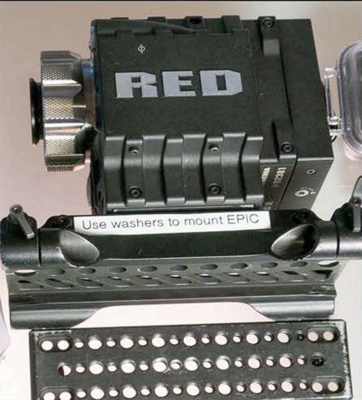
Epic Brain w. adapter plate and base plate, Cap for PL mount
